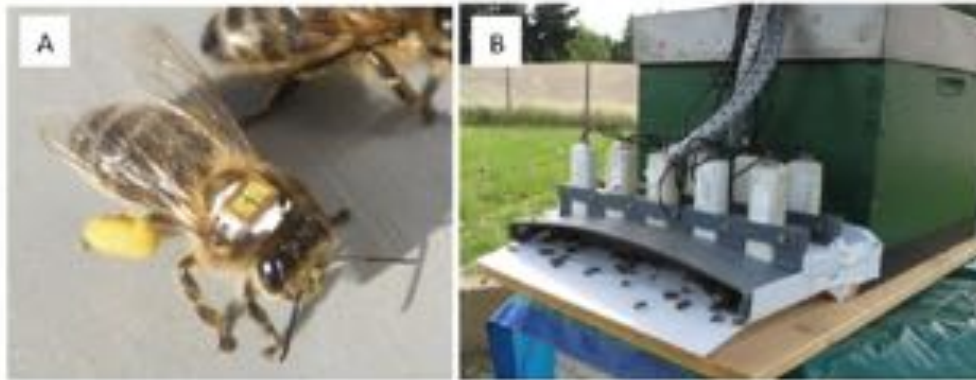
Fig. 1. Honey bee RFID monitoring equipment. (A) A pollen-forager honey bee fitted with a 3-mg RFID tag. (B) A hive entrance equipped with RFID readers for detecting returning marked foragers.
